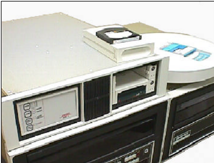
AEM-5C with Jaz disk and SCSI drive removed. DEC RK05 drives (lower) with removable cartridge - capacity 2.5 MB each.
