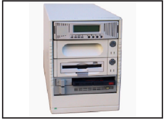
ASPX Emulation System mounted in a table-top cabinet. Unit is shown with control unit (top to bottom), removable SCSI hard drive, Magneto Optical drive, and Data Cassette tape drive. Unit is available with any combination of SCSI devices.
